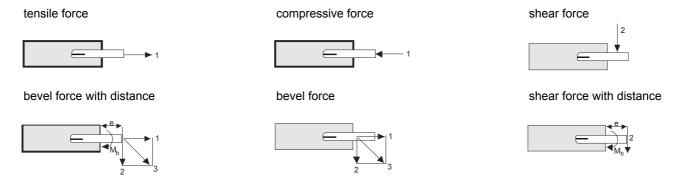
1= tensile/compressive force, 2= shear force, 3= resulting force, Mb= bending moment
